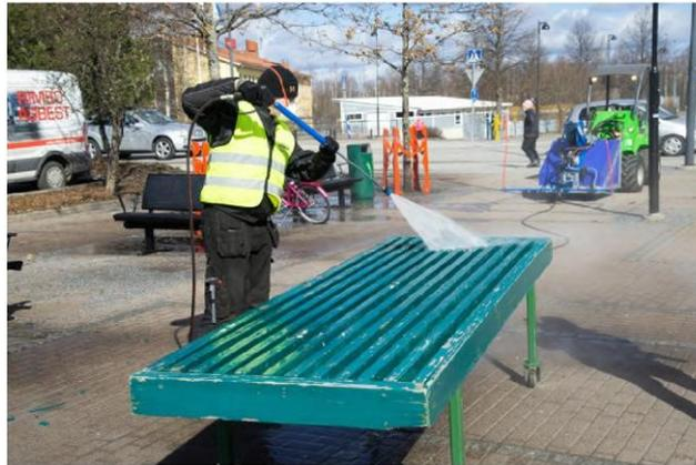
The flow of the power washer of the unit can be adjusted by adjusting the hydraulic oil flow of the pump. Another option is to swap the nozzle of the washing gun. This makes the power washing pistol a perfect disinfection tool. The same tricks work for the unit's washing boom also.
