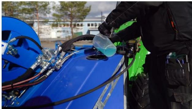
The disinfectant concentrate can be added directly to the container of the KPL Unit. Just measure the right dose of the concentrate, add fresh water to the container, and your disinfectant fluid is ready for use. This makes KPL a handy piece of disinfection equipment.
